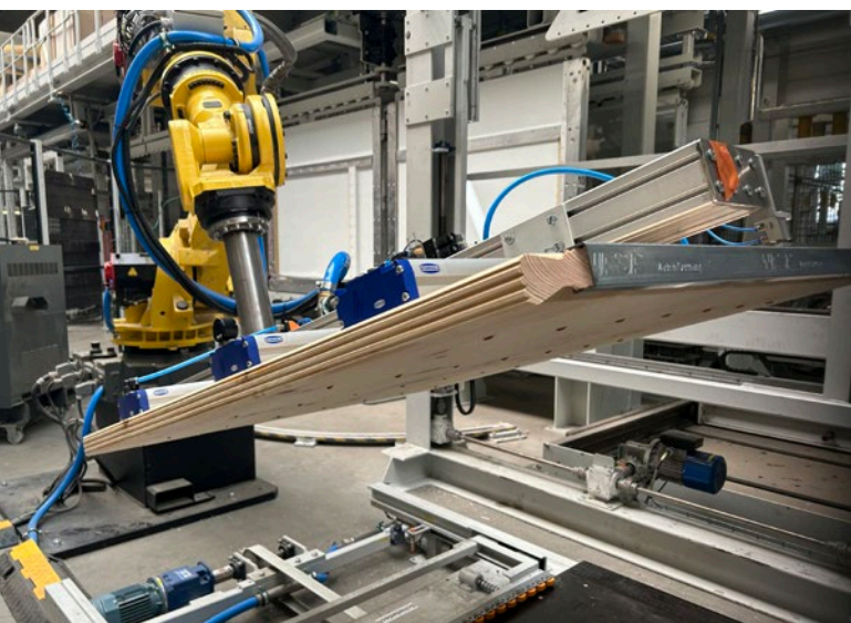
An industrial robot with a vacuum gripper picks up a wooden core and lifts it into another processing station, where spacers are also attached to the outer edges.
