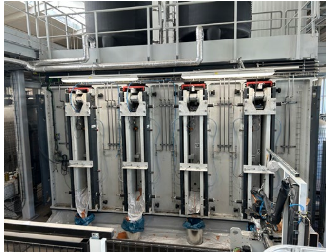
In the pressing stations, the liquid polyurethane is pressed into the mould at high pressure.
