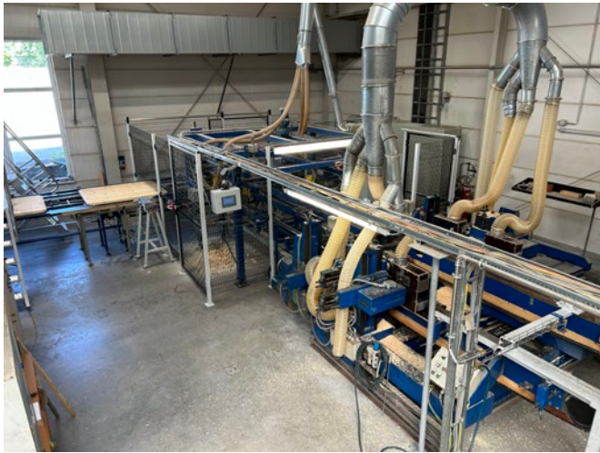
In several processing stations, the individual planks are first assembled to form a board and then milled at the corners and edges.
