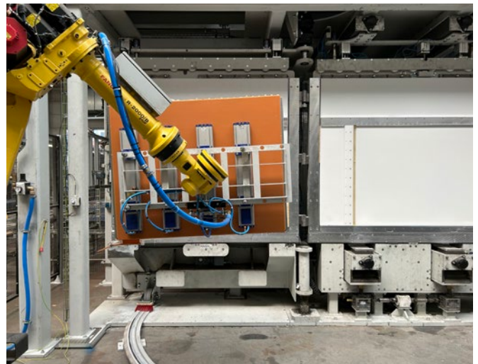
In the pressing stations, the liquid polyurethane is pressed into the mould at high pressure.
