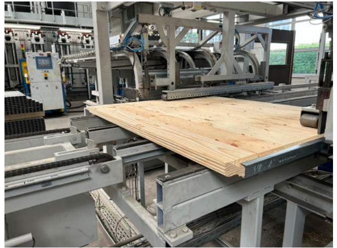
Wasa uses a 2 mm thick galvanised steel profile to fix the individual planks of a finished wooden core together.
