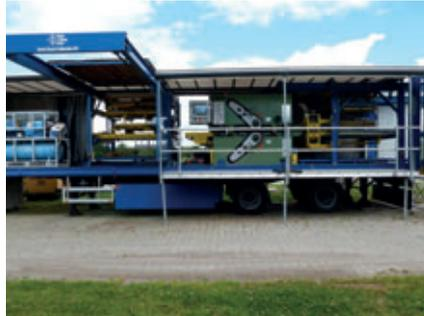
Wasa is extending its range of services for the calibration of production boards and now offers grinding on site at the customer's premises using truck-mounted grinding machines. Up to 4,000 boards can be ground on the top side and underside over a weekend. All the customer has to provide is space for the truck and a fork-lift truck.
