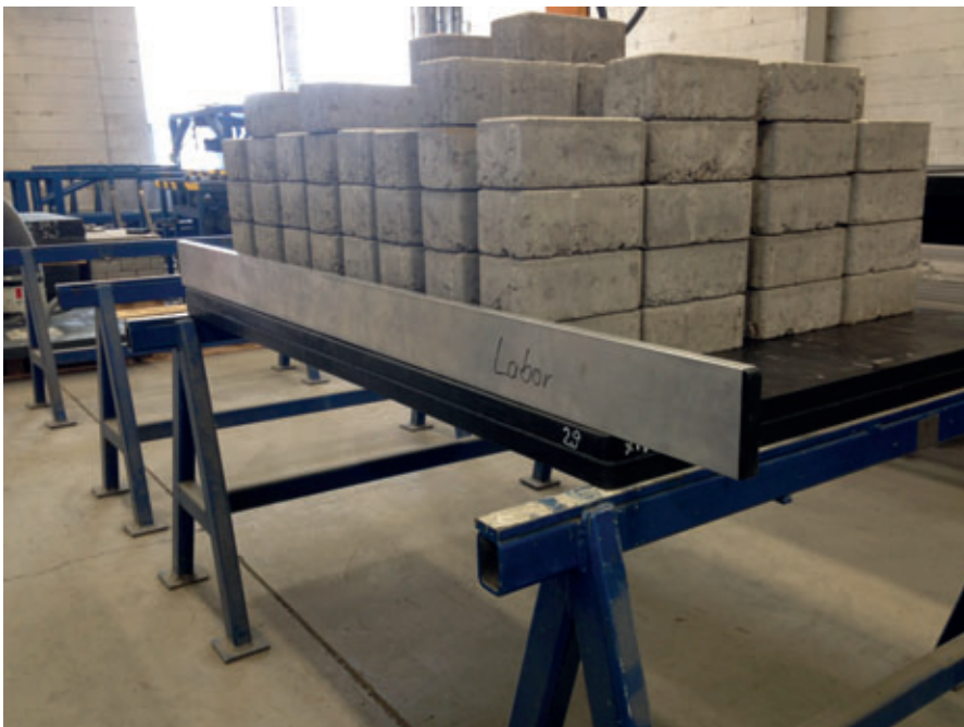
Due to the new structure of the Wasa Tecboard it was possible to triple the modulus of elasticity in comparison with the old Tecboard. It is now around 12,000 N/mm 2
