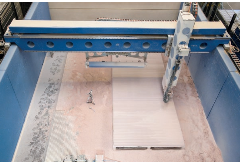
CNC machining of PU block material, model dimensions 3,600 x 1,500 mm. The structure is milled into the block material by a state-of-the-art 5-axis portal milling machine.
