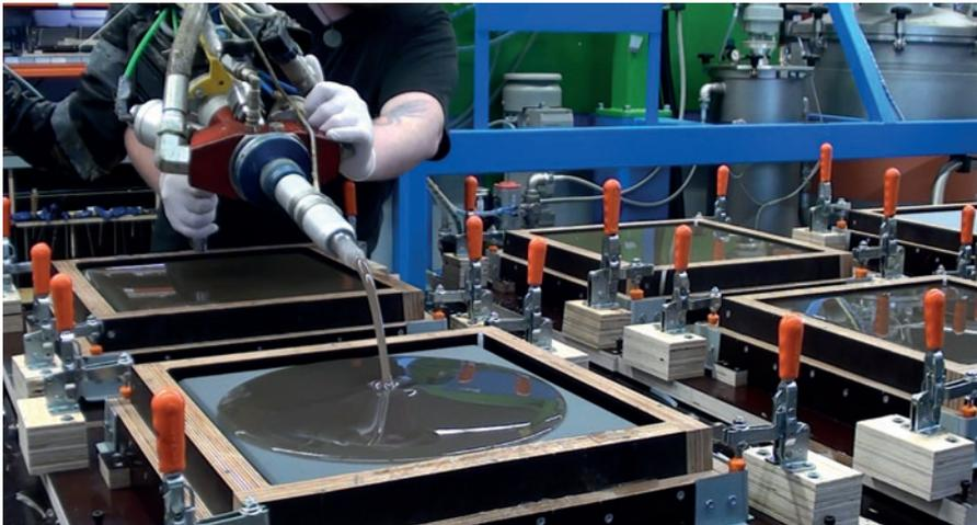
Insight into the manufacturing of high quality wet cast moulds with machine and computer-controlled technology
