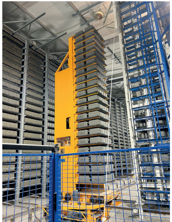
The hardening chamber of the new Quadra Q12 with Wasa Uniplast Ultra boards
