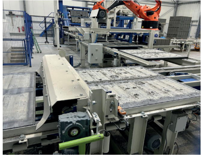
Thorough maintenance of the Wasa Uniplast Ultra through board cleaning in the Quadra Q12
