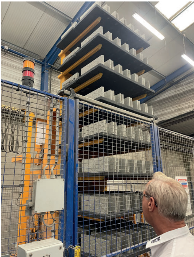
Quadra Q6 circulation system with Uniplast Ultra
