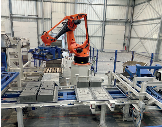
Robot handling in the modern circulation system of the Quadra Q12 machine
