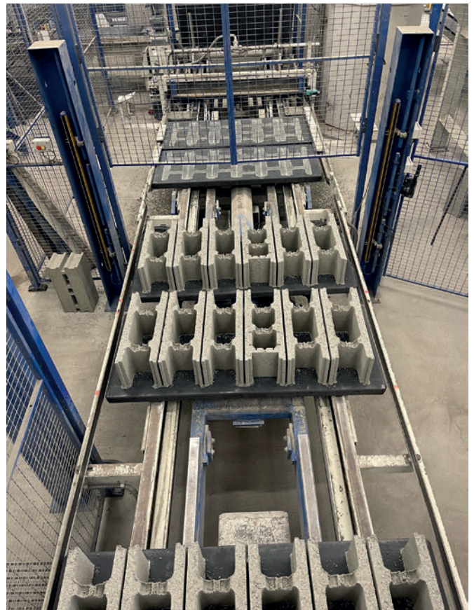
Very high compression and uniform height of the products due to the new solid plastic boards on the Quadra Q6
